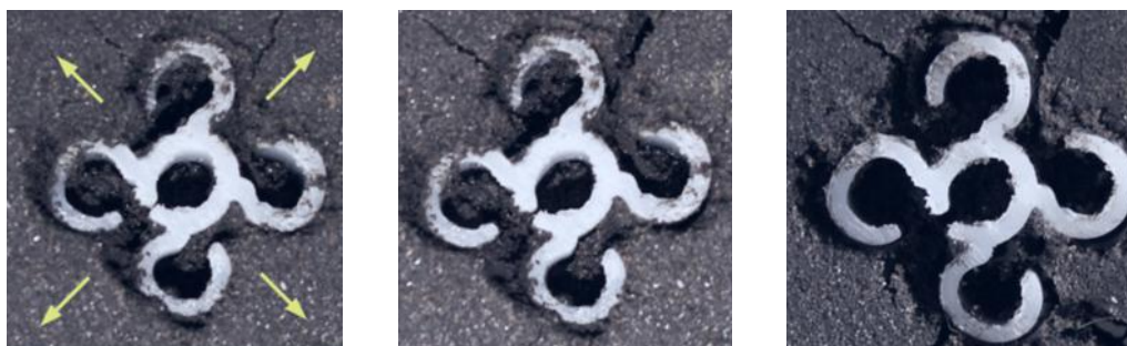
Figure 5 – Blades of a EXLTERRA GEPS unit opening when the soil is dry.
