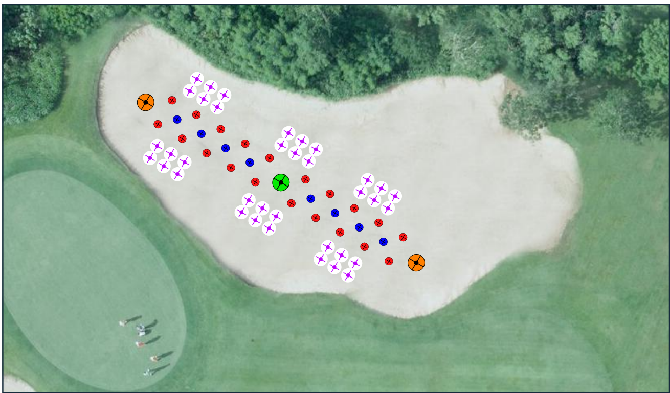
Figure 16 – A golf course bunker with EXLTERRA BSTR offline. EXLTERRA BSTR are on both sides of the EXLTERRA GEPS line because the water flow is entering the EXLTERRA GEPS line from two directions.
