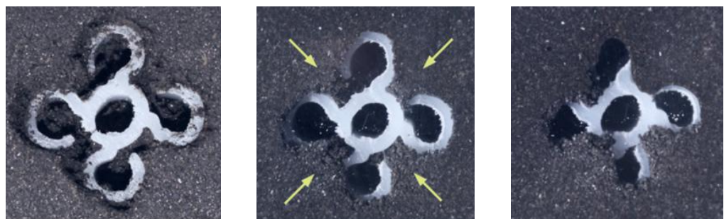
Figure 2 – Moist soil pushes the blades on the closed EXLTERRA GEPS unit.
