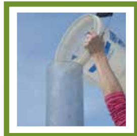
Figure 9: Filling Infiltrometer with Water
